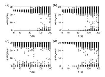
FIG. 10. The final orientation of a 24-atom flake (mapped onto the interval  $[0^{\circ}, 30^{\circ}]$ ), which was initially in the stable incommensurate periodic orbit is plotted as a function of temperature after a long, but finite time, with  $F_{\text{load}}=20$  nN,  $v_s=32$  m/s for scan lines (a) 1, (b) 2, (c) 3, and (d) 4. For every temperature, 250 realizations are plotted. Enough time has elapsed for the system to decay to the static state distribution.
