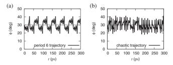
FIG. 3. Examples of more complicated trajectories of a 24-atom flake: (a) a periodic trajectory with a longer period, in this case 6 lattice periods, for  $F_{\text{load}}$ =30 nN at scan line 3 and (b) a chaotic trajectory for  $F_{\text{load}}$ =40 nN at scan line 1. All other conditions are the same as for the trajectories plotted in Fig. 2.
