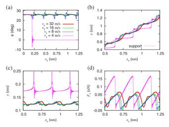
FIG. 12. (Color online) The (a) orientation  $\phi$ , positions (b) x and (c) y, and (d) friction  $F_s$  as a function of support position  $x_s$  for various support velocities and N=24,  $F_{\text{load}}=20$  nN, scan line 2. As the velocity decreases, the fluctuations in  $\phi$  and y increase and the system behaves less one-dimensionally. For sufficiently low  $v_s$ , the system can no longer be described by the simplified model.
